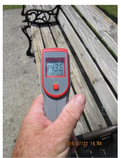
Image 7: Forest Drive Columbia transit bus stop bench..wooden planks over cement base..143.6°
